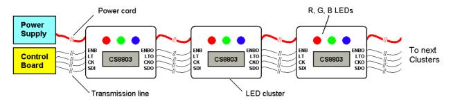
Fig.1 The typical structure of LED cluster signage
