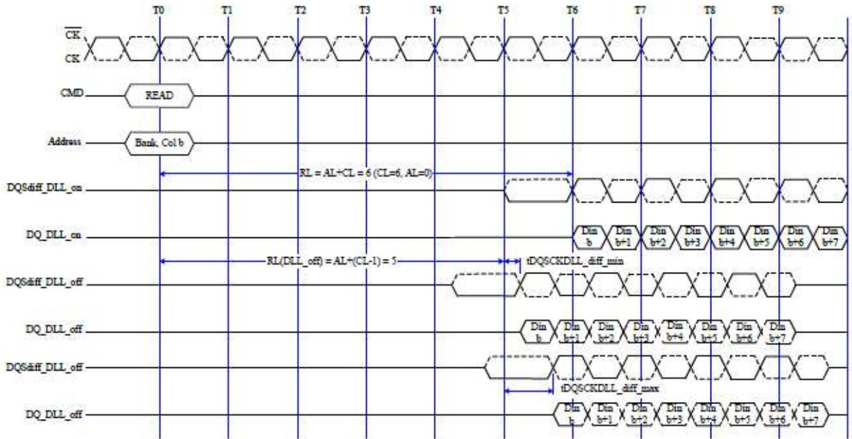
Note: The tDQSK is used here for DQS,  $\overline{DQS}$ , and DQ to have a simplified diagram; the DLL\_off shift will affect both timings in the same way and the skew between all DQ, DQS, and  $\overline{DQS}$  signals will still be tDQSQ.
