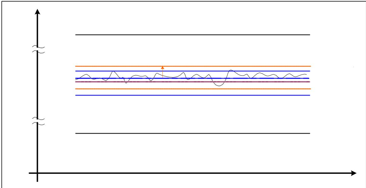
**DDR3 Differential AC and DC Input Levels for clock (CK -  $\overline{\text{CK}}$  ) and strobe (DQS -  $\overline{\text{DQS}}$  )**
