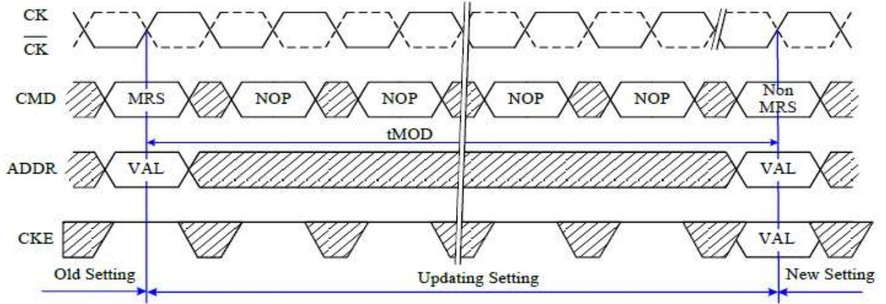
The mode register contents can be changed using the same command and timing requirements during normal operation if the DRAM is in idle state, i.e., all banks are in the precharged state with tRP satisfied, all data bursts are completed, and CKE is high prior to writing into the mode register. The mode registers are divided into various fields depending on the functionality and/or modes.
