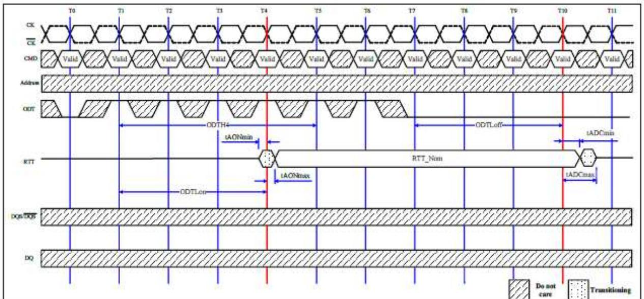
Note: ODT<sub>H4</sub> is defined from ODT registered high to ODT registered low, so in this example ODT<sub>H4</sub> is satisfied; ODT registered low at T<sub>5</sub> would also be legal.
