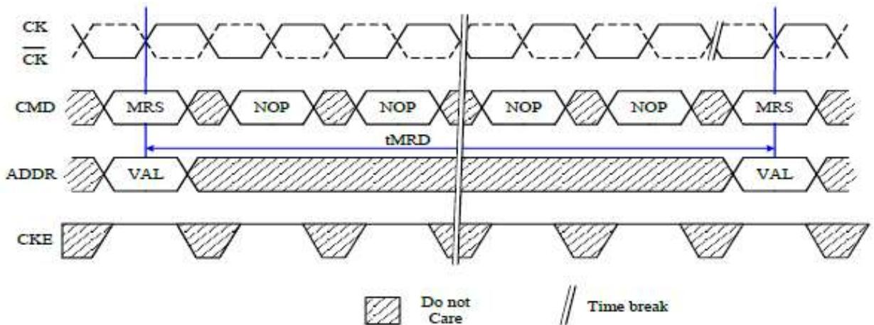
The MRS command to Non-MRS command delay,  $t_{MOD}$ , is required for the DRAM to update the features except DLL reset, and is the minimum time required from an MRS command to a non-MRS command excluding NOP and DES shown as the following figure.
