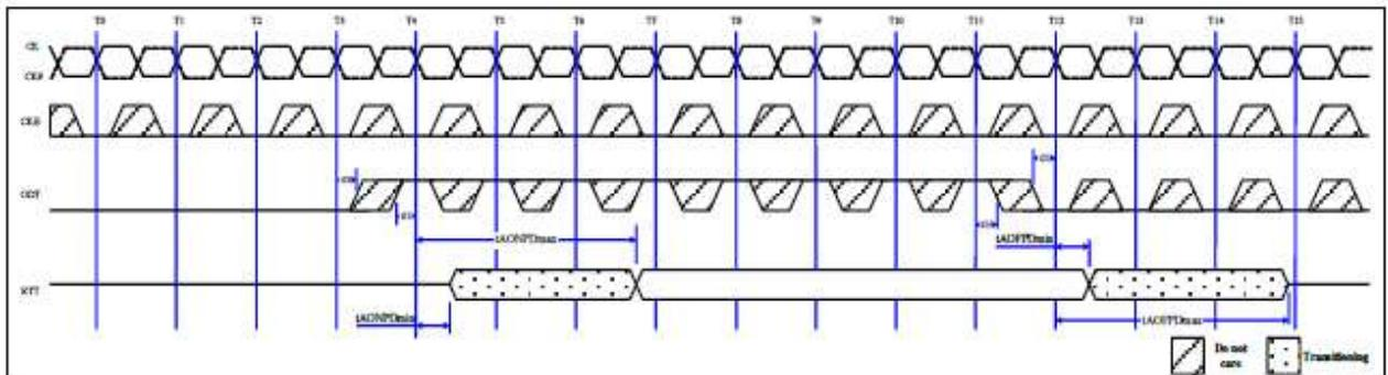
In Precharge Power Down, ODT receiver remains active; however, no Read or Write command can be issued, as the respective ADD/CMD receivers may be disabled.
