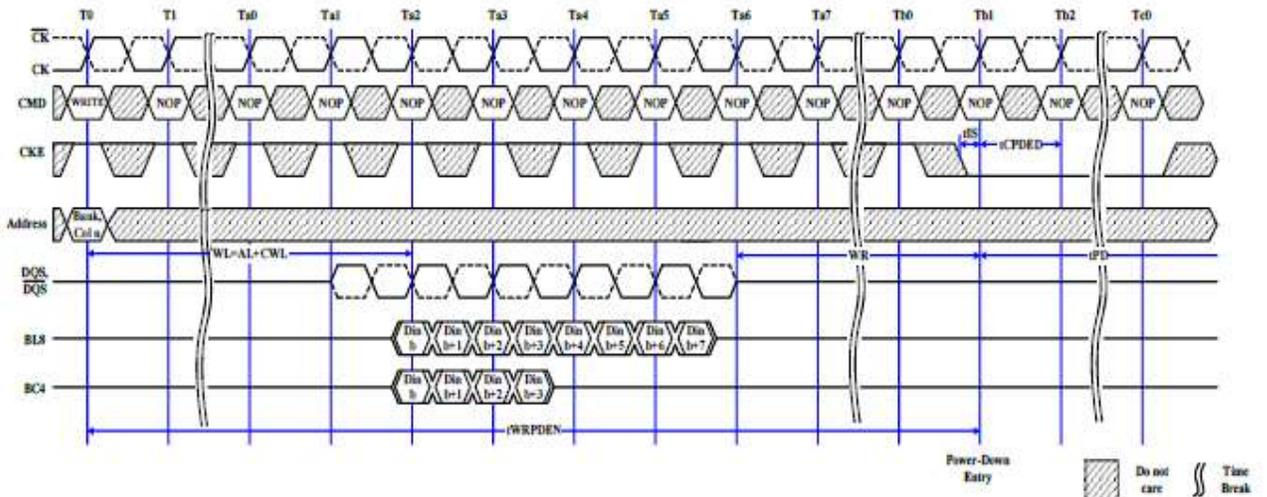
**Precharge Power-Down (Fast Exit Mode) Entry and Exit**
