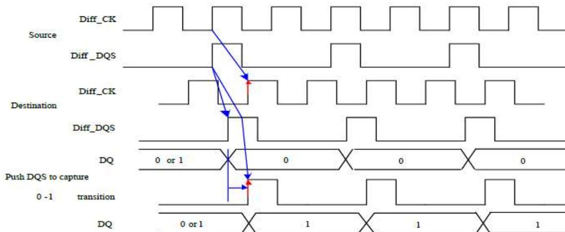
$\overline{DQS} - \overline{DQS}$  driven by the controller during leveling mode must be determined by the DRAM based on ranks populated. Similarly, the DQ bus driven by the DRAM must also be terminated at the controller.
