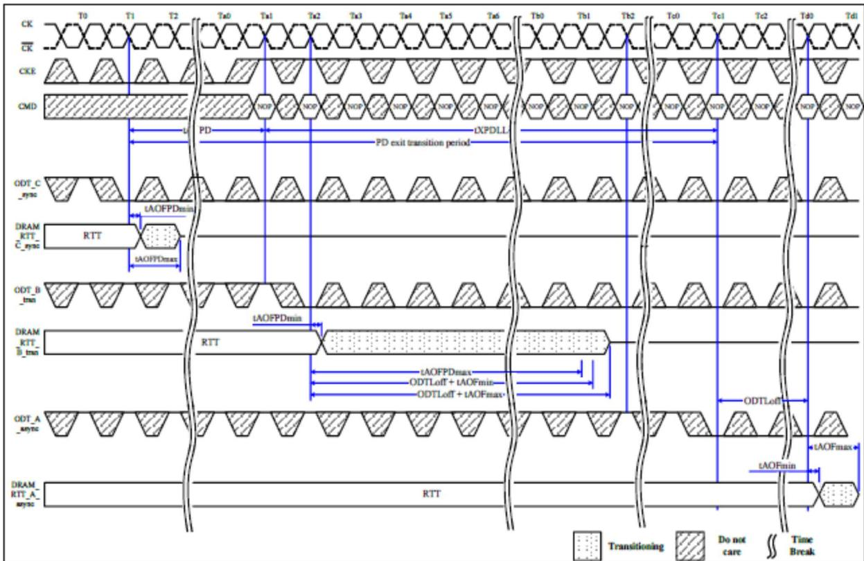
**Asynchronous to Synchronous ODT Mode during short CKE high and short CKE low periods**
