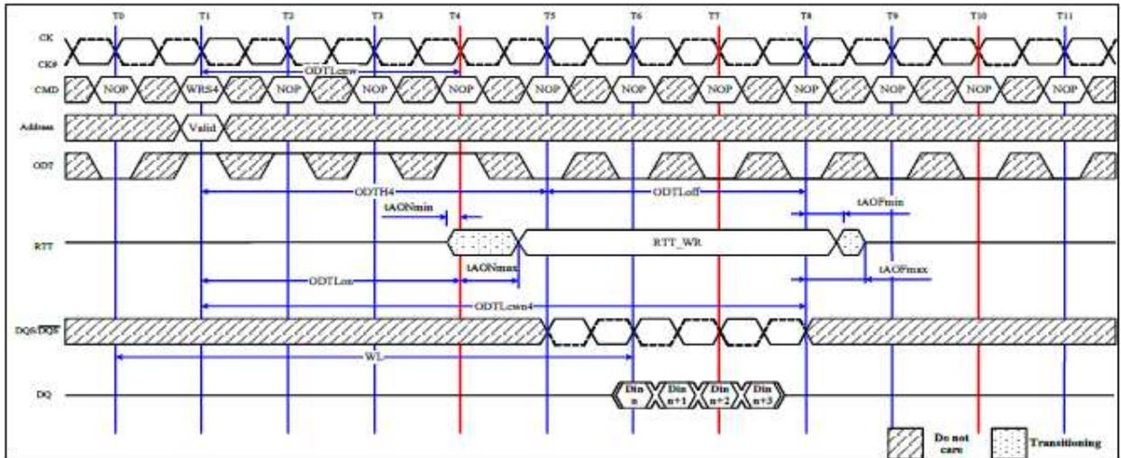
**Asynchronous ODT Mode**
