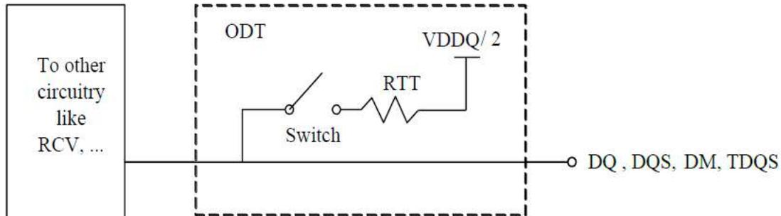
The switch is enabled by the internal ODT control logic, which uses the external ODT pin and other control information. The value of RTT is determined by the settings of Mode Register bits. The ODT pin will be ignored if the Mode Register MR1 and MR2 are programmed to disable ODT and in self-refresh mode.
