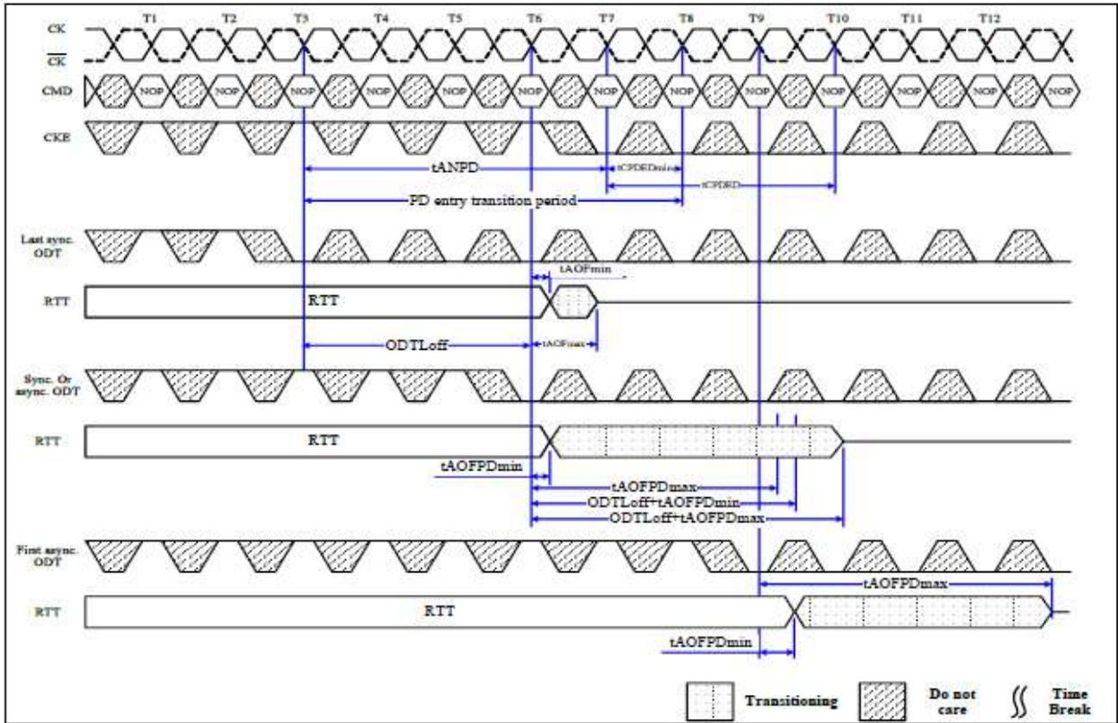
**Asynchronous to Synchronous ODT Mode transition during Power-Down Exit**
