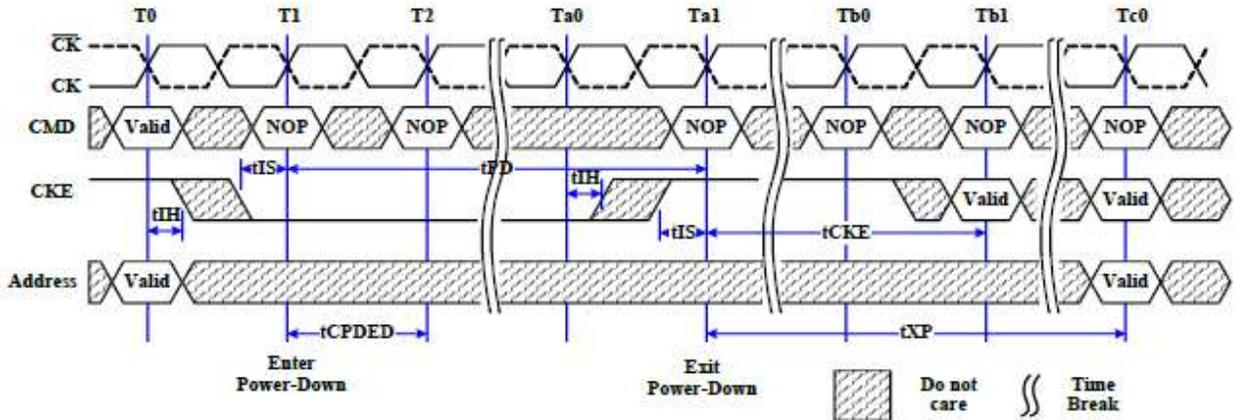
Timing Diagrams for CKE with PD Entry, PD Exit with Read, READ with Auto Precharge, Write and Write with Auto Precharge, Activate, Precharge, Refresh, MRS:
