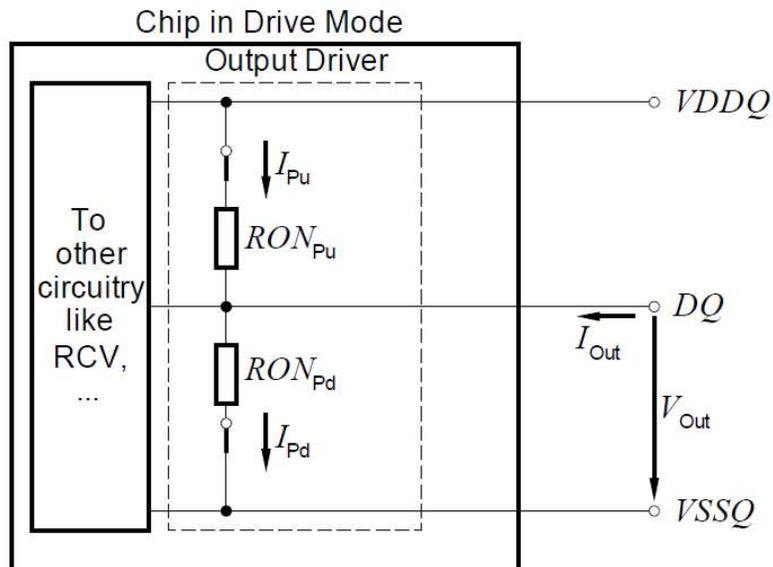
Output Driver DC Electrical Characteristics, assuming  $R_{zQ} = 240\text{ohms}$ ; entire operating temperature range; after proper ZQ calibration
