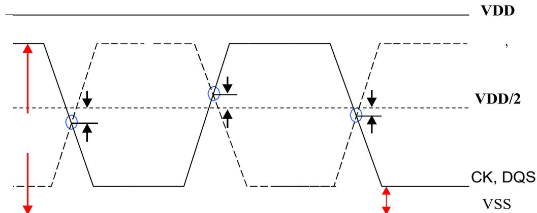
**Cross point voltage for differential input signals (CK, DQS)**
